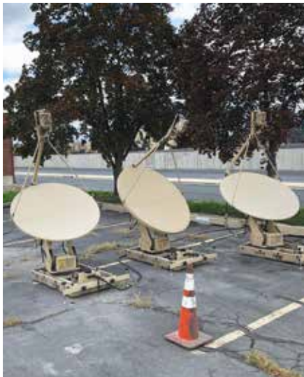
The G4 SASMO section sets up multiple VSAT systems outside Draper's Combined Support Maintenance Shop as part of the migration process to the Sustainment Tactical Network ensuring their operability on the new network.
