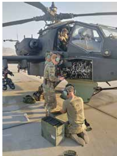
The 1-211th ARB crew chiefs' re-arm the AH-64 following aircraft maintenance in Mazar-e-Sharif, Afghanistan.
